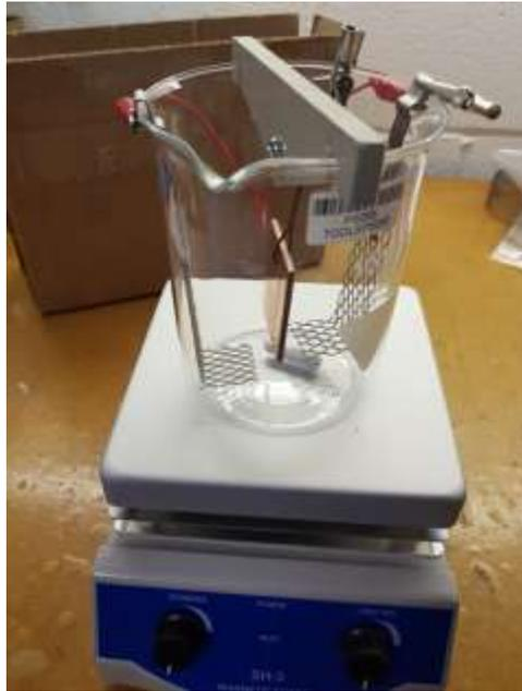
**Plating cell showing two inert mesh anodes and a central copper cathode**
