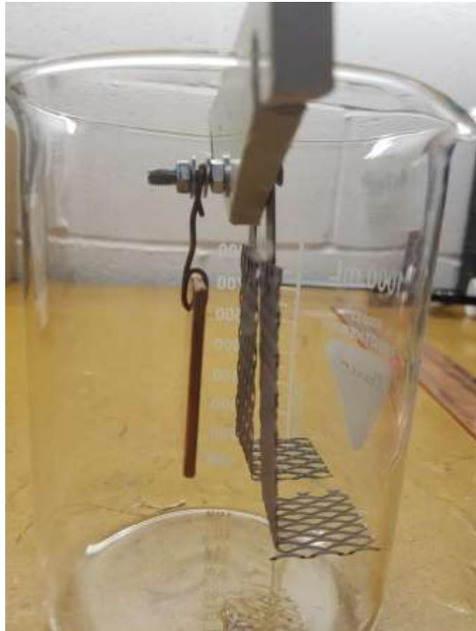
**Anode to cathode spacing reduced to 1 cm**
