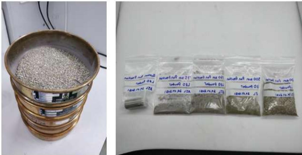
Figure 16. Fractionation of ball-milled powder, filter cans (left) and fractionated powders (right).
