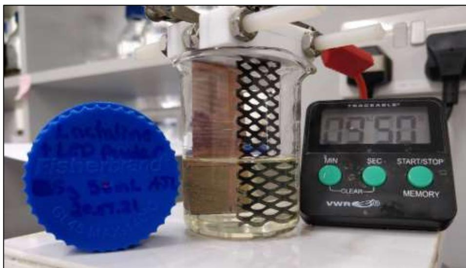
**Figure 12.** Experimental set-up for electrowinning from the Lactaline DES during electrolysis and showing clear colouration on the electroactive region of the Cu cathode.
