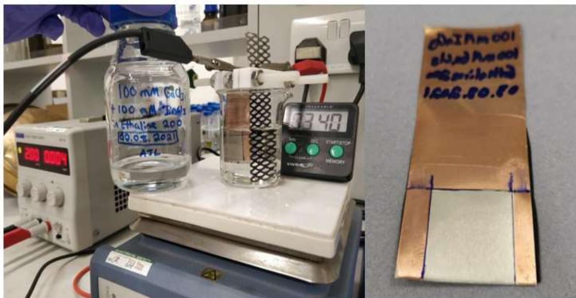
**Figure 17. Experimental set up for the test recovery of both In and Ga from a model DES solution containing 0.1 M  $\text{GaCl}_3$  and 0.1 M  $\text{InCl}_3$  in Ethaline 200 (left), Ga/In coated cathode piece (right).**
