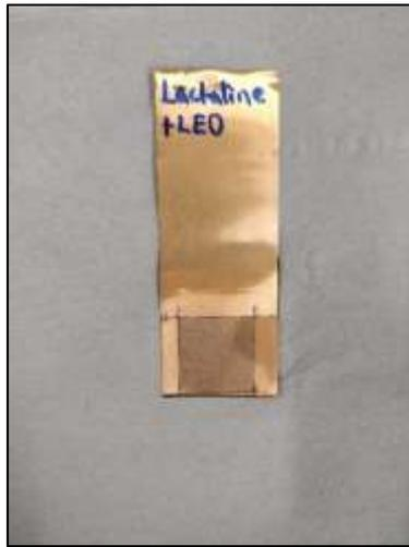
**Figure 13. Cathode piece removed from initial electrowinning experiment shown in Figure 12 having been rinsed in DI water and dried.**
