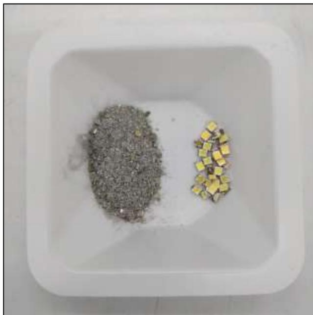
**Figure 9. LED chips from dismantled light lamps (right) and ball-milled powder (left).**
